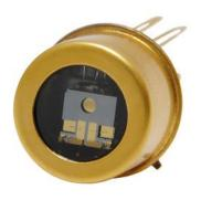
The CPOD serials cooled extended InGaAs photodiode provides ultra-low noise for detecting near-infrared light in the 1.2-2.6 µm range. These detectors are hermetically sealed to ensure longevity. Within the detector package, a thermoelectric cooler is integrated with options of 1, 2, and 3 stages, as well as integration with a MEMS chopper, significantly reducing background noise while maintaining a compact format. Additionally, a driving PCB with an amplifier is available for convenient use.
